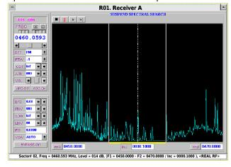
A priority-search operation allows the user to quickly step through a list of predefined signals. The user may enter up to 100 frequencies into a priority-search list. During the priority search, bar-graph displays assist in monitoring the status of each signal. As with the spectral search, the user can tune the receiver by pointing to the desired signal on the display.
