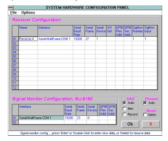
With the system-hardware configuration panel, an operator can easily alter system-setup or create multiple system-configuration files in advance and later download them for quick system changes.
