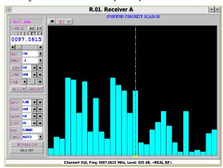
Programmable report-actions and lockout functions supplement the search operation. The report-actions function supports search for new signals, search for all signals, or skip all adjacent signals. The lockout function allows an operator to exclude RF spectrums from the spectral-search operation. The operator may define up to 200 lockout segments. The user may define lockout segments by frequencies and bandwidth, or by Start and Stop lockout frequencies.
