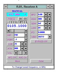
Control Rxs may provide up to 12 receiver-control panels, each fully independent and tailored to accommodate the receiver. The panels offer four different types of control operations. A simple and easy-to-use manual operation allows the user to monitor and change manual-tuning receiver parameters.
