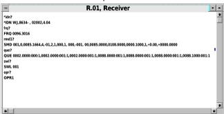
In addition to the four different operational types, Control Rxs also provide access to a signal-list editor window. The user may enter information such as tuned frequencies, IF bandwidth, COR setting, detection mode, signal identification, and comments. The user can then use the information from the list to create a priority-search list for the priority-search operation, a lockout list for the lockout function, and a hand-off signal for the hand-off operation.
